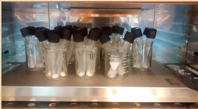
Fig. 2 Set up for enzymatic digestion of sieved material
